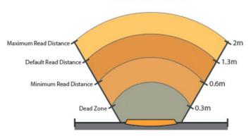
Radar detection range. Spanning from a 60° FOV from the e-loop, these are the range zones. The Gray area depicts the dead zone, in which objects cannot be detected. The Minimum read distance is 0.6m. The default read distance is 1.3m, and the Maximum read distance spans up to 2m.
