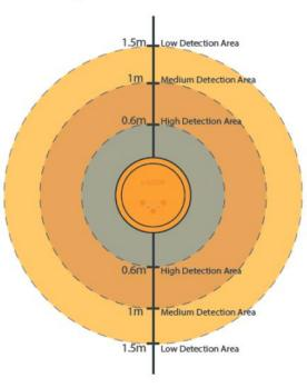
Varying magnetic field detection zones. The grey area depicts a 0.6m high sensitivity detection area surrounding the e-loop, suitable for the majority of vehicles. The dark colour area depicts a 1m medium sensitivity detection area surrounding the e-loop, suitable for most vehicles. The light colour depicts a 1.5m low sensitivity detection area surrounding the e-loop, which is only suitable for some vehicles.
